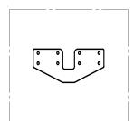
Reinforcement brackets in structure joints.
