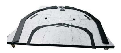
3°. Start assembling the side walls and archs. Now the walls and floor perimeter can be fixed to the platform.
